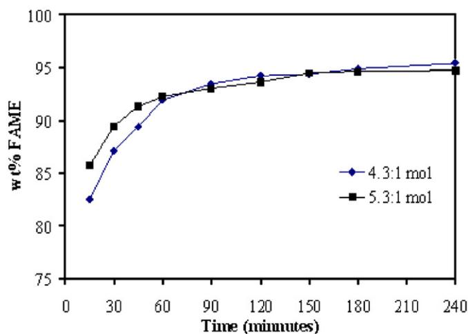
Fig. 3. Effect of reaction time on FAME content at 90 °C, 4.3:1 and 5.3:1 molar ratios of methanol to PFAD and 1.834 wt% of H<sub>2</sub>SO<sub>4</sub> under its own pressure.
