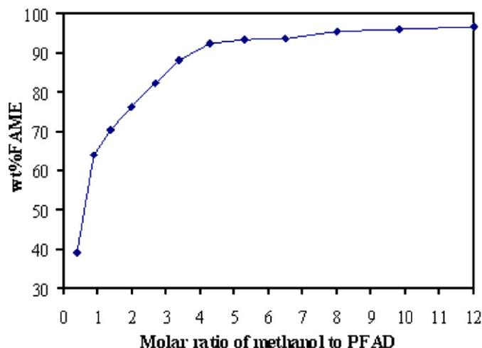
Fig. 2. Effect of molar ratio of methanol to PFAD on FAME content at 90 °C, 4 h and 1.834 wt% of H<sub>2</sub>SO<sub>4</sub> under its own pressure.
