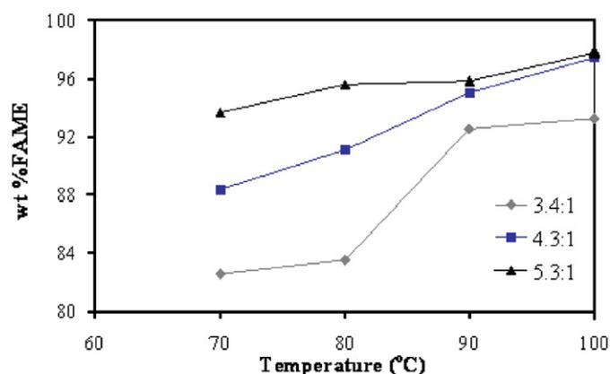
Fig. 4. Effect of reaction temperature on FAME content at 3.4:1, 4.3:1 and 5.3:1 molar ratios of methanol to PFAD, 2 h and 1.834 wt% of H<sub>2</sub>SO<sub>4</sub> under its own pressure.
